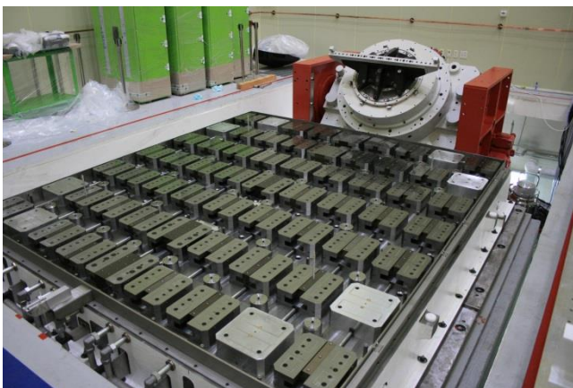
Slip table without large plate (bearings view)
