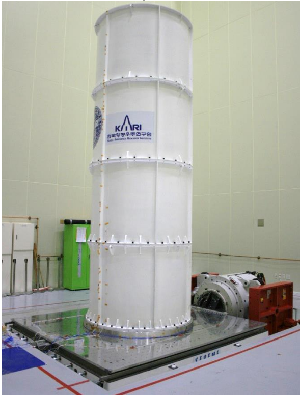
Slip table in large configuration with 11 tons KARI dummy
